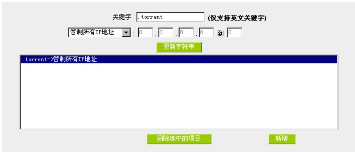
The screenshot shows the 'Content Filtering' configuration page. At the top, there is a search bar labeled '关键字 : .torrent (仅支持英文关键字)' with a note '(仅支持英文关键字)'. Below it is a dropdown menu '管制所有IP地址' followed by a range selector '到' with four input fields for IP addresses. A green '更新字符串' button is located below the range selector. A blue header bar displays the text ',torrent->管制所有IP地址'. At the bottom, there are two buttons: '删除选中的项目' (Delete selected item) and '新增' (Add new).
